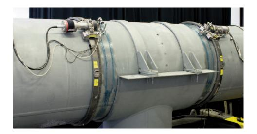
Multiskip can be used on both pipes and plate, and is suitable for inaccessible geometries such as clamps, saddles and pipe supports. This eliminates the need for expensive shutdown and lifting of equipment by providing information that allows integrity decisions to be made. Sonomatic offers a full service to customers in carrying out Multiskip inspections for a range of situations.
